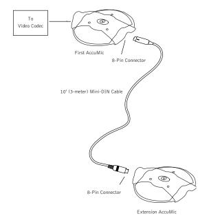
Figure 16. Connecting an AccuMic VC Extension Mic
